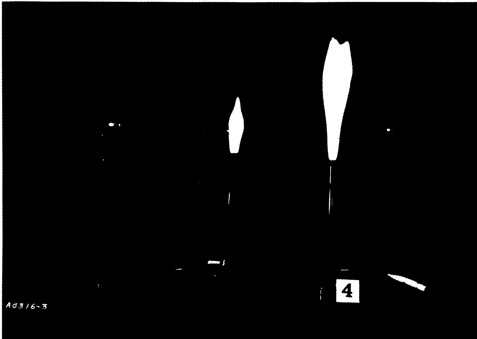
Flames burning from glass tubes showing the halo around the flame. No voltage applied.
